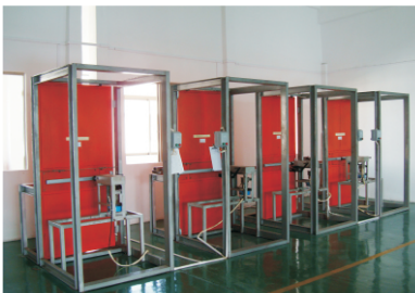
6. Test machine for panic exit device 8 set , According to EN1125 U1305
