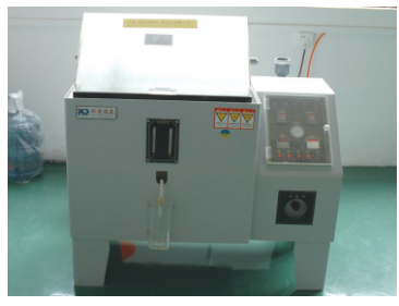
5. Test machine for security lock furniture 1 set , According to EN1906
